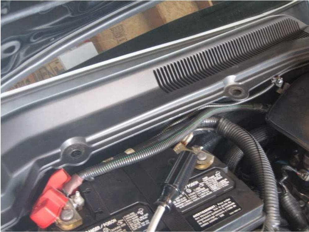
Carefully lift up the cover to expose the cabin air filter.
