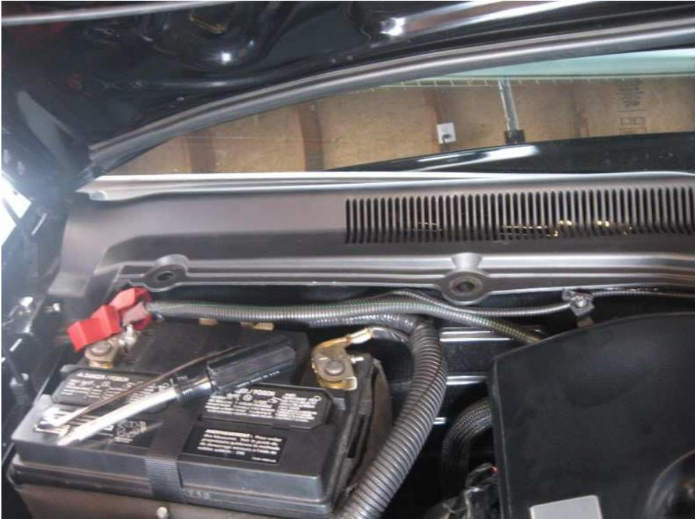
Make sure the cover is positioned back into the original location. The cover seal should sit flush up against the windshield.
